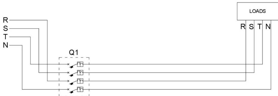
Pre-installation diagram without ICO-F system
